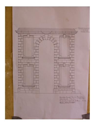
The central range was brought forward once more, in the form of a meticulously designed and academic Palladian elevation. The surviving south wall of the medieval hall was exposed to the elements once more behind a giant order semi-circular arch in the centre of the range.
